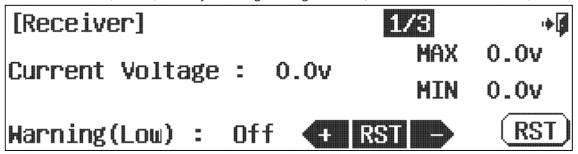
d. Additional voltage sensor screen (up to 100v) which is available when using the "Electric" Sensor Station (HTS-SS Blue).
