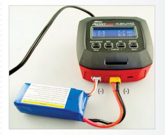
This diagram shows how to correctly connect your battery to check the internal resistance.
