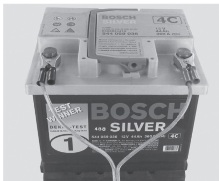
Using alligator terminal clips attached to a car battery.
