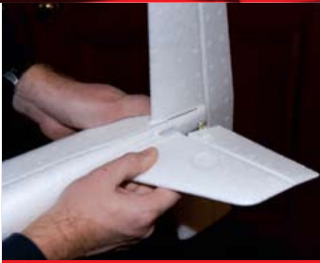
▲ The way the parts are molded makes installing the tail feathers very simple. This is a model that goes together quick and easy because of prefabrication.
