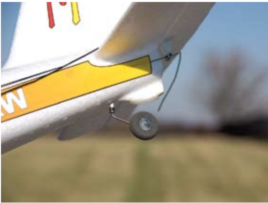
▲ The tailwheel addition is a must as far as I'm concerned. It is easy to do and makes the MiniMag a lot more fun on the ground.
