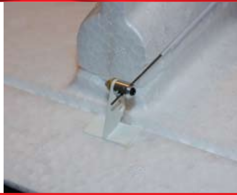
▲ You just guide the pushrod through the barrel and lock down the screw after making sure the elevator is properly centered.
