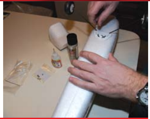
▲ One of the few assembly steps involved in getting the RTF version ready involves snapping the landing gear wire into place and screwing in a retaining bolt.
